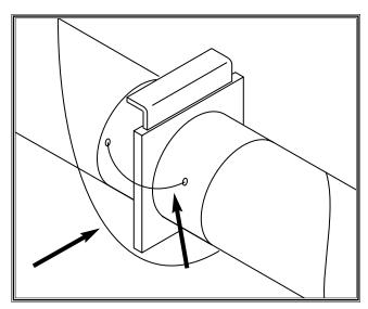
Figure 20. Ground wires bypassing blast gate.
